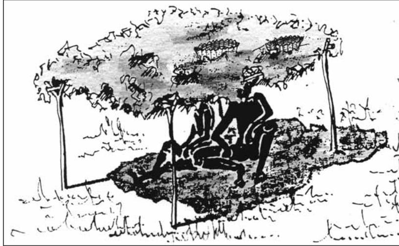
**Figure 2.5** A flat-roof shade *barabar*, constructed of four forked posts and cross-rails.
